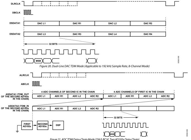
Figure 21. ADC TDM Daisy-Chain Mode (256 f<sub>5</sub> BCLK, Two AD193x Daisy Chain)
