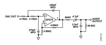
Figure 31. Typical DAC Output Filter Circuit (Single-Ended, Noninverting)
