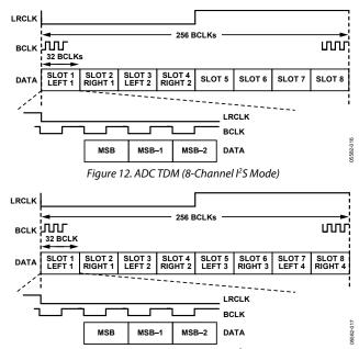
Figure 13. DAC TDM (8-Channel I<sup>2</sup>S Mode)
