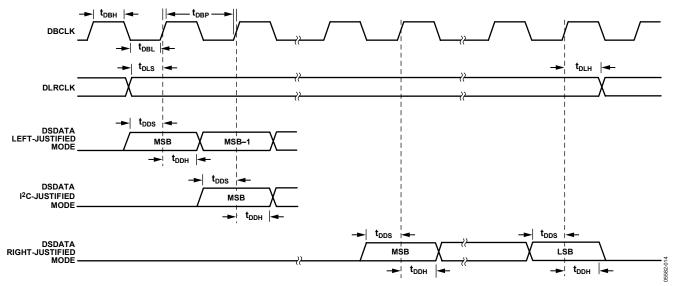
Figure 24. DAC Serial Timing
