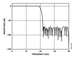
Figure 6. DAC Stop-Band Filter Response, 48 kHz
