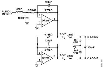
Figure 29. Typical ADC Input Filter Circuit
