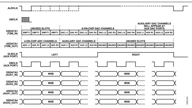
Figure 17. Combined AUX DAC and ADC Mode
