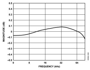
Figure 9. DAC Pass-Band Filter Response, 192 kHz
