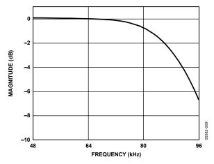
Figure 10. DAC Stop-Band Filter Response, 192 kHz
