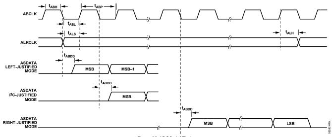
Figure 25. ADC Serial Timing
