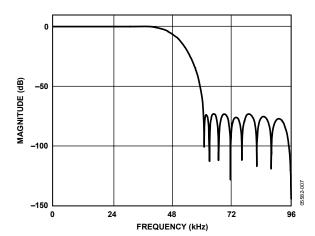
Figure 8. DAC Stop-Band Filter Response, 96 kHz
